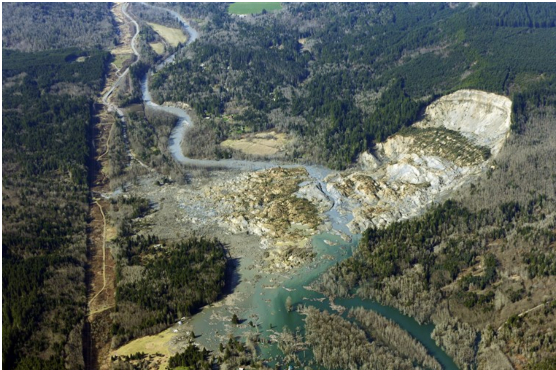
The town of Oso used engineering to prevent a bend in the North Fork Stillaguamish River from migrating to the left in the photo, fearing it would flood and/or erode the town. However, the river ended up steepening the base of the slopes to the right, thus contributing to the 2014 Oso landslide.
